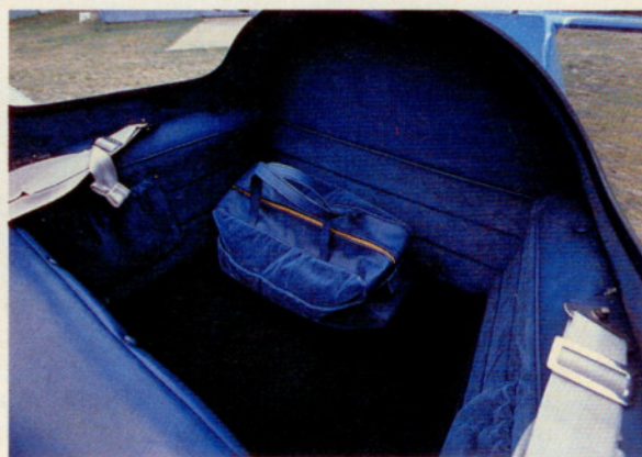
A storage shelf behind the seats can hold up to 65 pounds of gear. Shadoan installed four-point harnesses for added safety.
